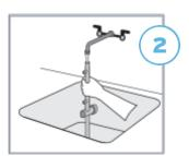
Unscrew wash arms and end caps. Flush under running water. Clean nozzles with toothpick. Remove soil inside the pre-wash and wash tank area of dishmachine using a brush, water and **manual detergent**. Insert parts back into dishmachine.
